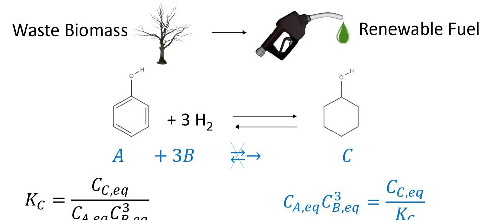
$K_C$  >2000 at room temperature, I could not detect the reverse reaction, or any reactants at equilibrium (X  $\approx$  1 at equilib.). However, at ~300 °C,  $K_C$  is only ~0.03! Exothermic
